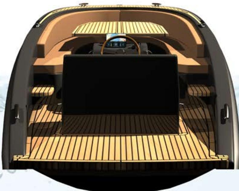
The flush deck and weather proof cushions provide impressive hose-and-go readiness. The one-handle control and bow thruster (option) make the AY-800 easy to maneuver and its polyurethane fender bars provide the AY-800 with great protection without the hassle of normal fenders.
